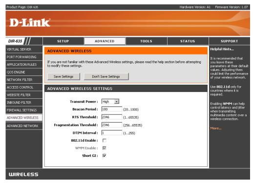
**802.11d:** This enables 802.11d opration. 802.11d is a wireless specification developed to allow implementation of wireless networks in countries that cannot use the 802.11 standard. This feature should only be enabled if you are in a country that requires it.
